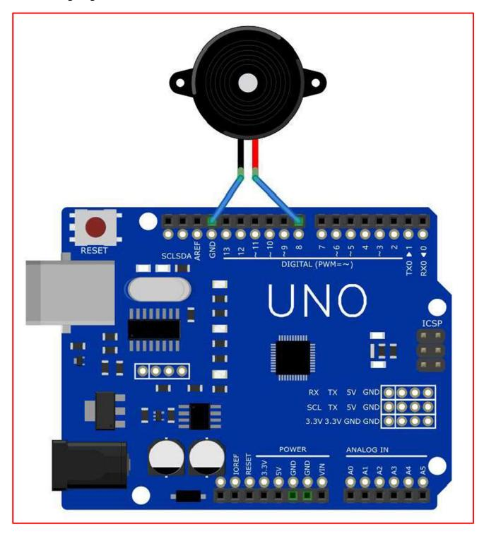
Wiring the buzzer connected to the UNO R3 board, the red (positive) to the pin8, black wire (negative) to the GND.
