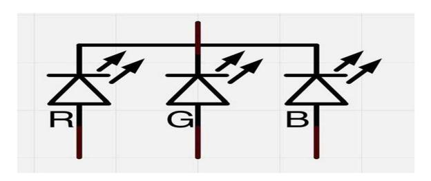
Here on the photographs you can see 4 electrode LED. Every separate pin for Green or Blue or Red color is called Anode. You will always connect "+" to it. Cathode goes to "-"(ground). If you connect it other way round the LED will not light.
