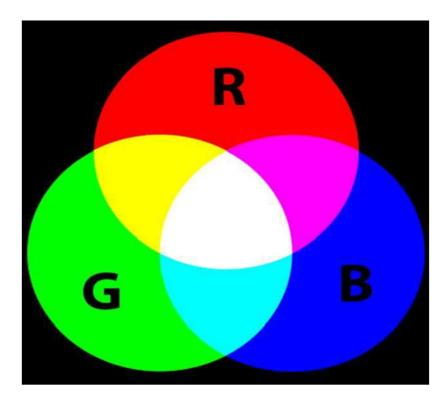
If we set the brightness of all three LEDs to be the same, then the overall color of the light will be white. If we turn off the blue LED, so that just the red and green LEDs are the same brightness, then the light will appear yellow.
