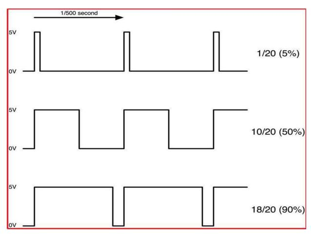
Roughly every 1/500 of a second, the PWM output will produce a pulse. The length of this pulse is controlled by the 'analogWrite' function. So 'analogWrite(0)' will not produce any pulse at all and 'analogWrite(255)' will produce a pulse that lasts all the way until the next pulse is due, so that the output is actually on all the time.
