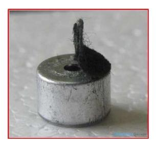
A solid conducting metal body encapsulates the various parts of the microphone. The top face is covered with a porous material with the help of glue. It acts as a filter for the dust particles. The sound signals/air vibrations passes through the porous material and falls on the diaphragm through the hole shown in the image above.
