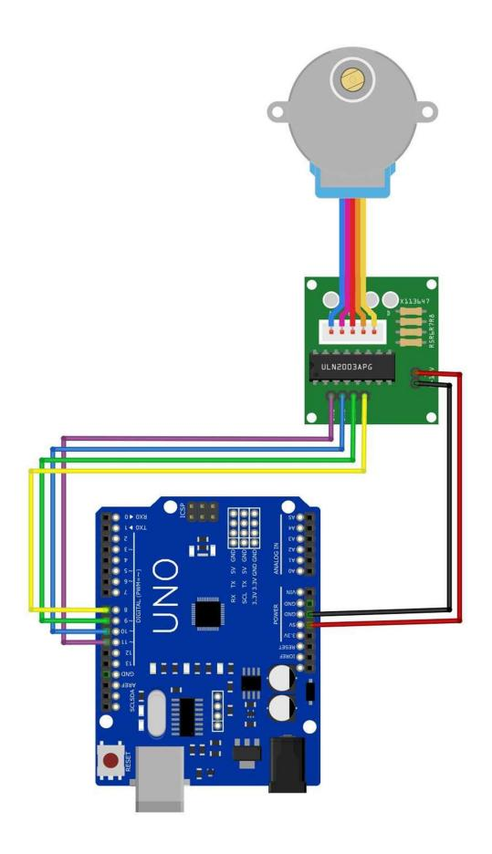
We are using 4 pins to control the Stepper. Pin 8-11 are controlling the Stepper motor.
